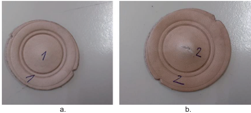
Figure 1 Leather samples after testing the resistance to cracking: a. sample VEG; b. sample VEG +Z
