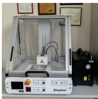
Figure 1 Spraybase® melt electrospinning device
