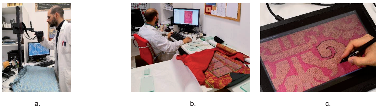
Figure 1 Various techniques used for digitising historical textile patterns: a. photographing with adjustable copy stand; b. recording on a flatbed scanner; c. applying graphic tablet for tracing the pattern
