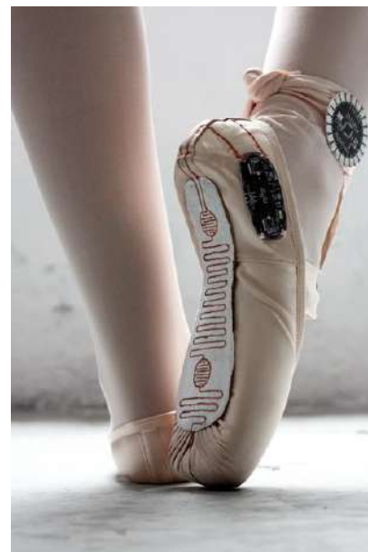
Figure 7: Ballet slippers with embedded microcontroller [11]
