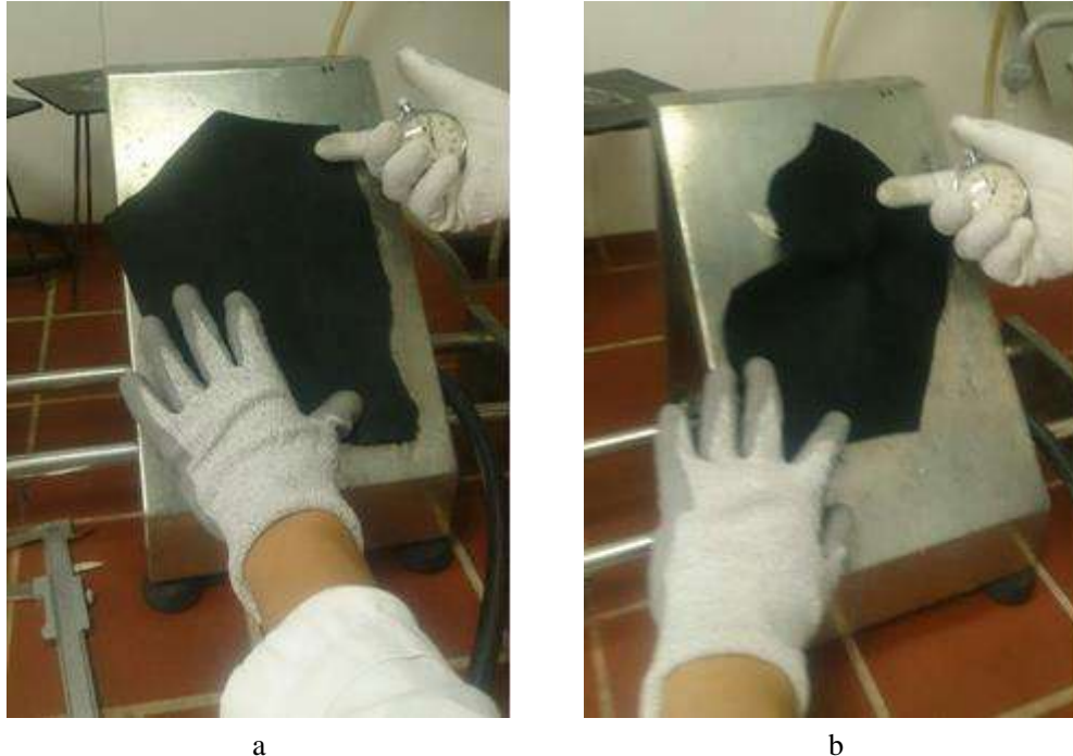
Figure 2: Burning process according to HRN EN ISO 15025: 2003
