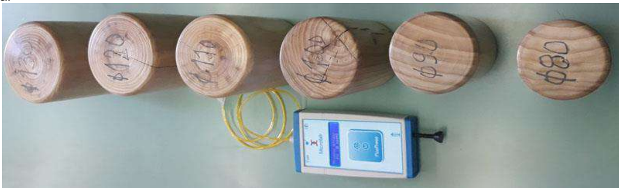
Figure 2: Wooden cylinders with diameters of 80 do 130 mm and PicoPress device for measuring sock compression
