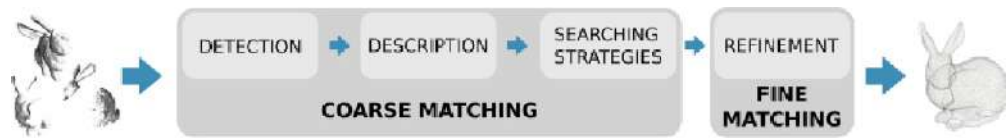
Figure 2: Pipeline of the detection-description-matching approach. Taken from [13].
