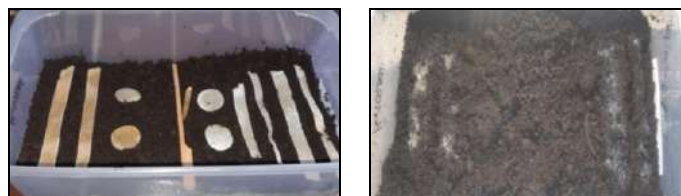
Figure 7: Samples before and after burial in the ground
