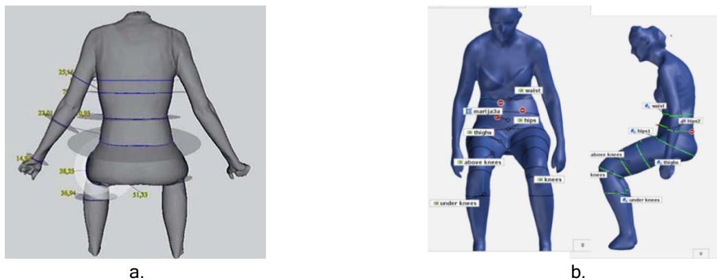
Figure 2: Definition of measurements on a 3D point cloud of the human body in sitting position (a- back side, b- front and lateral side) [17, 18].
