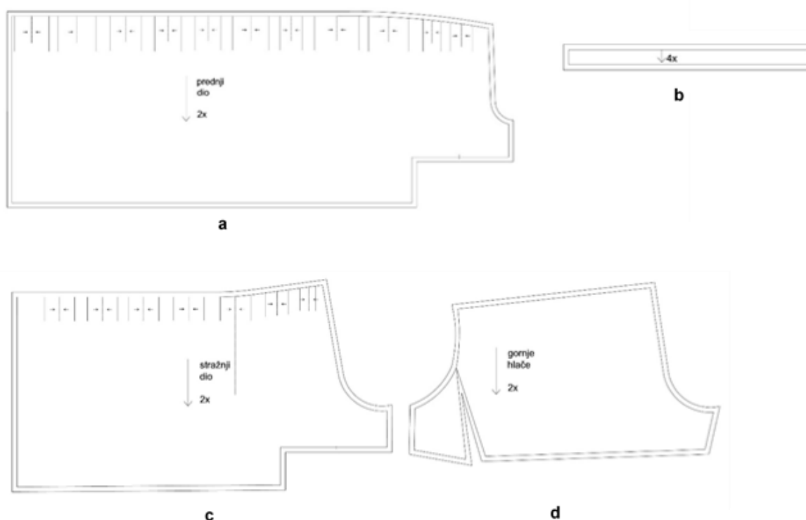
Figure 4: Modeled patterns of the garment: a) second part of inner trousers, front, b) belt, c) one out of two parts of inner trousers, back, d) outer trousers
