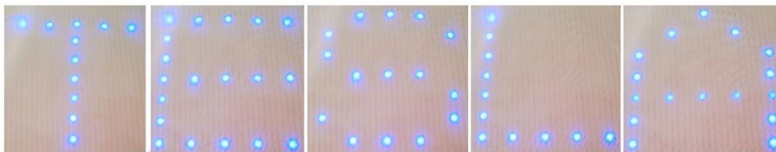
Figure 12: Remote control on the LE diode matrix with the word TESLA printed on it
