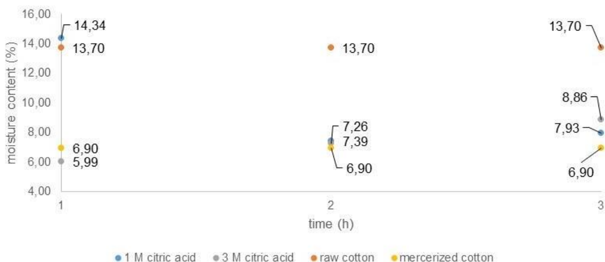
Figure 2: Moisture content of cotton samples modified with grafted gelatine and citric acid.
