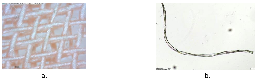
Figure 4: The dress is made of breathable and lightweight cotton fabric ( etamine ): a. Macro photography of the plain weave of the cotton fabric taken with a Dino lite digital microscope, b. Longitudinal microscopic image of the warp
