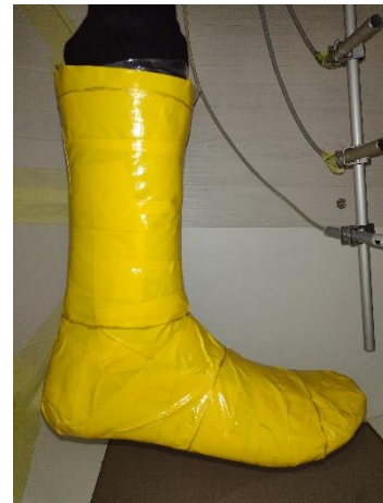
4c: Fabric backing electrical tape is used to reinforce the plastic shrinkwrap, mold the shape of the foot; and transfer the elastic band markings onto it
