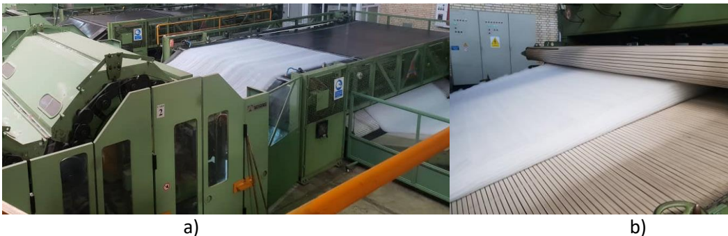
Figure 7: a) The main cylinder of carding machine b) the web that created in output of the cross lapper consisted of 10 layers
