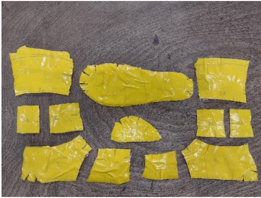
4d: After unmolding, the form is cut open along the elastic band markings and the contour of the shape; then numbered
