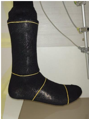
Figure 4a: The base sock (sweating layer) is on the thermal foot, and elastic bands are used to divide the foot into sections for unmolding and patternmaking
