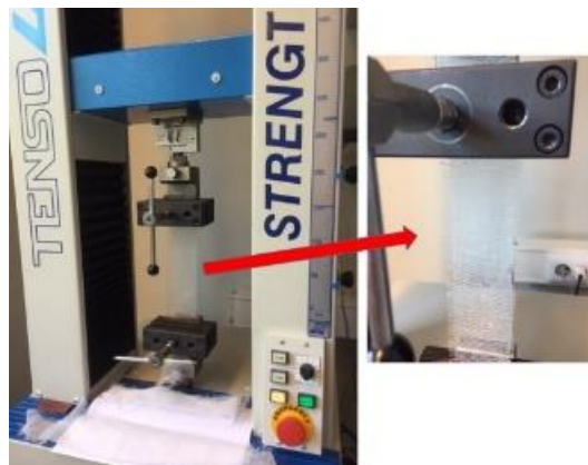
Figure 2: Appearance of the test sample in the clamps prepared for testing
