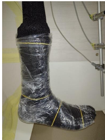
4b: A plastic shrinkwrap is applied to cover the entire foot model
