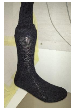
Figure 2: A 100% wetted cotton sock is put on the thermal foot model as the sweating layer
