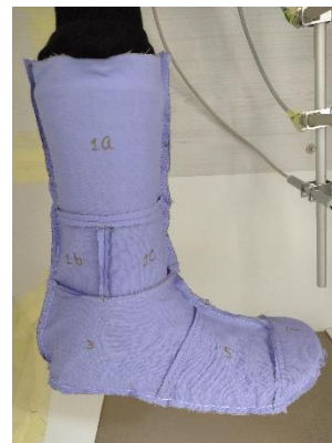
4g: After the cut and sew process, material pattern pieces are turned into a 3D sock that is ready to be tested
