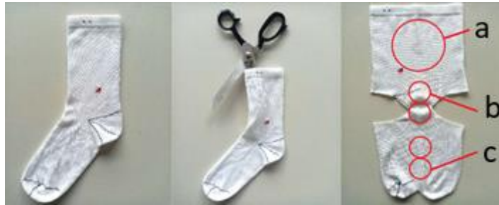
Figure 1: Sampling of socks: a) for testing of propensity to surface pilling; b, c) for testing of abrasion resistance
