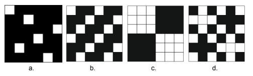
Figure 1. Construction weaves of selected fabrics: sample: a. Atlas 5/1; b. Twill 2/1 Z; c. Regular Panama 3/3; d. Kanava
