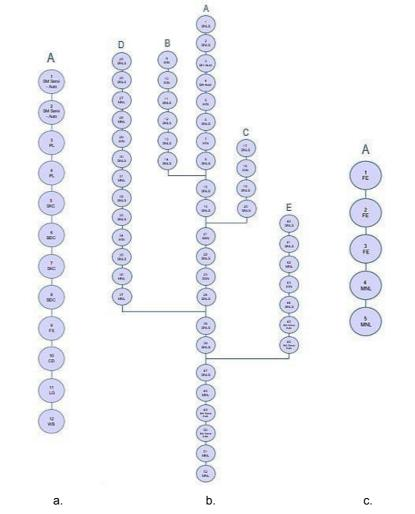
Figure 1: Flow chart of technological operations for a. cutting, b. sewing, c. finishing of a men's shirt
