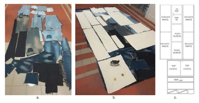
Figure 1: Work process - zero waste pattern on reused denim - top and pants; a. art composition, b. cutting plan, c. patterns
