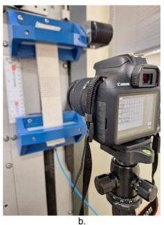
Figure 1: Measuring system: a) schematic view: 1) upper clamp; 2) lower clamp; 3) fabric sample; 4) light source; 5) remote control; 6) testing machine; 7) camera; 8) macro lens; 9) slider; 10) tripod, b) photo
