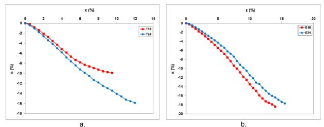
Figure 3: Diagram of relative contraction of fabric s (%) when force acts: a) in weft direction, b) in warp direction
