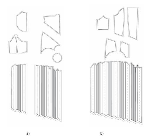
Figure 4. Tailoring parts of the a) front and b) back with seam allowance
