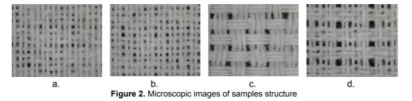
The structure of the samples is observed, also, by digital microscope imaging. The microscopic images are shown in Figure 2.
