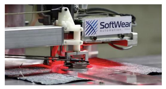
Figure 3: SoftWear's sewing robot that can handle the textile material, position it correctly and sew.
