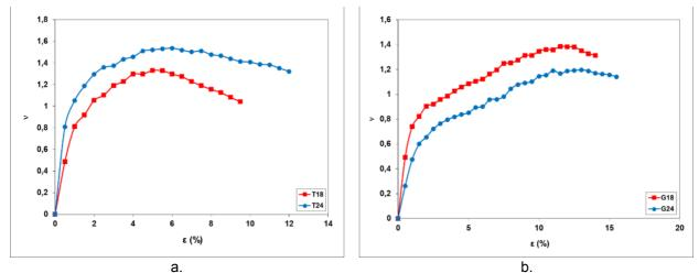
Figure 4. Poisson's ratio of the fabric v when the force acts: a) in weft direction, b) in warp direction
