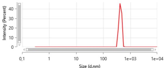
Figure 5: Size and distribution of silver nanoparticles after preparation of samples
