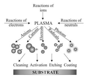
Figure 1: Plasma–substrate interactions [5]
