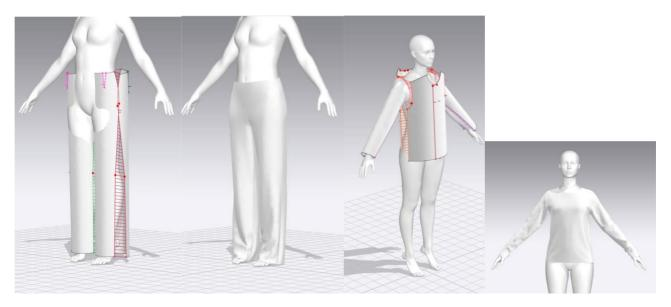
Figure 3: Virtual testing of the fit of the basic pattern of digital clothing with the computer program Clo 3D [1]
