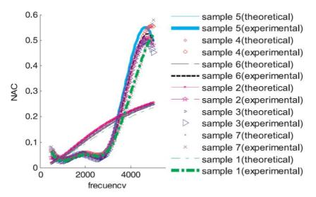
Figure 2: The fluctuations in the Noise Absorption Coefficient (NAC) across various frequencies in samples featuring varying quantities of knit and miss stitches, based on experimental and theoretical data [13]
