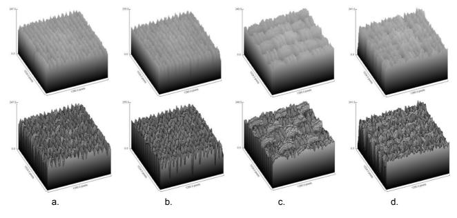
Figure 4: Surface Plot of the fabric samples: a. Atlas 5/1; b. Twill 2/1 Z; c. Regular Panama 3/3; d. Kanava from ImageJ program
