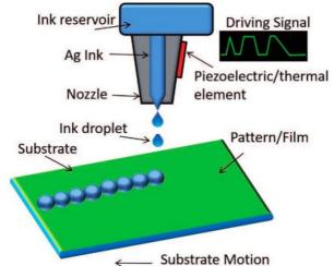
Figure 2: Schematic illustration of inkjet printing technology [18]
