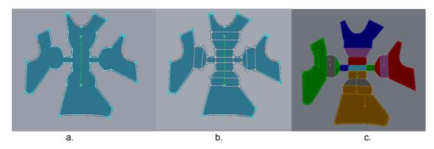
**Figure 2:** Digital process of spatial modeling form: a. digitalization of pattern, b. selection on small rectangle elements, c. separation on small patterns in the Modaris CAD Lectra system.
