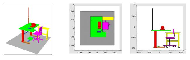
a. b. c. **Figure 1:** Designed workplace for the technological operation bartacking the seam on the sleeves, length and shoulder using the ERGOMas module: 3D view (a), blueprint (b) and side view(c).
