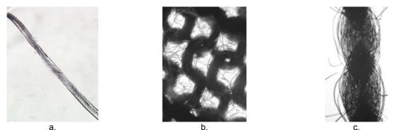
Figure 2. Microscopic figures of cotton – a. fiber under enhancemet 100x times; b. knitted fabric under enhancemet 4x times; c. yarn in woven fabric under enhancemet 40x times
