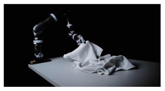
Figure 4: Sewts' robot, designed to perform advanced textile handling for various tasks
