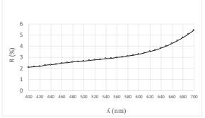
Figure 2 Graphic representation of the remission of the measured sample
