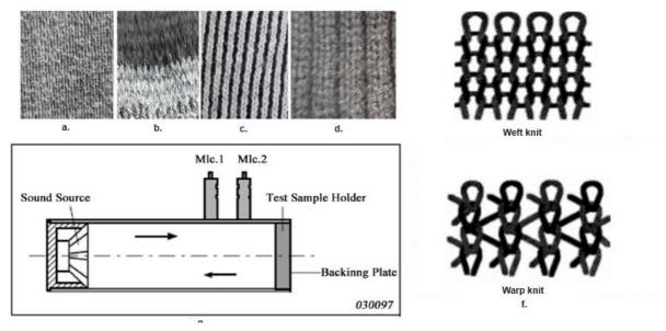
**Figure 1:** Specimens used for acoustic test, a nature fiber, b & c manmade fibers and blended fibers, e & f type of knitted fabric structure where e. represents weft knit, f represents warp knit, g drawing model of acoustic properties test with impedance tube [11]
