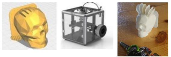
a. b. c. **Figure 3:** 3D printing: a. model of skull head with plate with holes for stitching made in Cura, b. creality sermon D1 3D printer, c. printed head compared to standard keys
