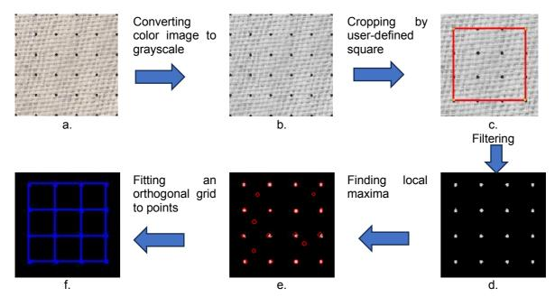
**Figure 2:** Stages of image processing and analysis and the resulting images: a) input image; b) grayscale image; c) image cropped; d) filtered image, e) local maxima on filtered image, f) best fitted to the regular grid in the first image.
