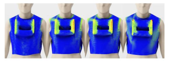
Figure 9: Warp elongation in the fabrics: F1, F2, F3, XCAD.
