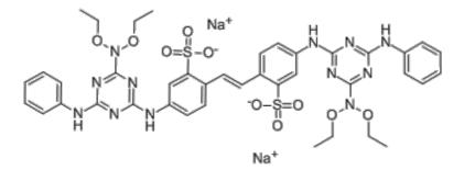
Figure 2: Uvitex BHT (CI Fluorescent Brightener 113) [5]
