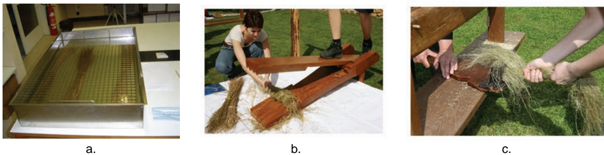
Figure 1: a) Laboratory retting of flax, b) mechanical extraction of fibres by crushing the stems on a stamping mill, c) combing the fibres
