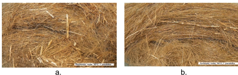
Figure 2: Flax fibres with nonfibrous cellulose material for samples: a) RBK I, b) Laura I
