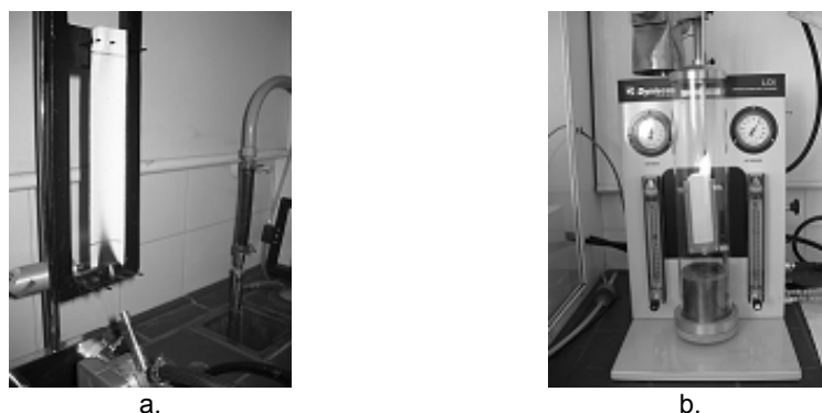
Figure 2: Equipment - a. Vertical test with possibility of surface and bottom edge ignition, b. LOI Chamber
