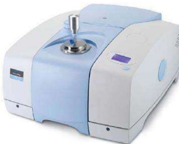
Slika 6: Spectrum 100 FT-IR (Fourier Transform Infrared) spektrometar, Perkin Elmer , USA
