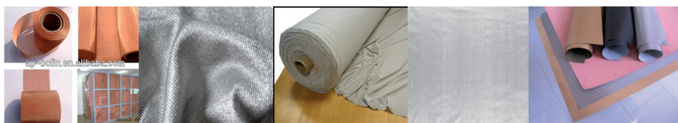
Figure 1 Interlinings materials with metal coatings against EM radiation [8]
