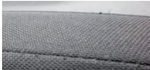
Figure 2 Woven fabric damage at the seam area appearing by using car seat cover
