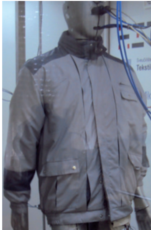
Figure 1 Intelligent clothing on the thermal manikin
