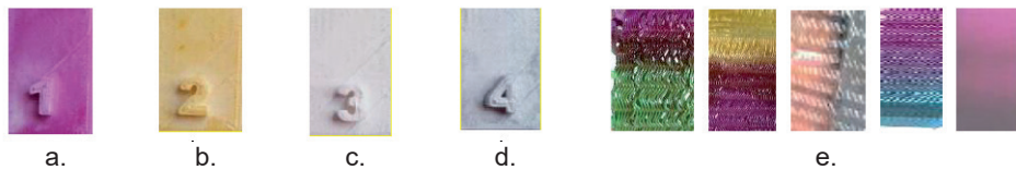
Figure 2 Coloured 3D samples by exhaustion process: a) dispersion colouring, b) acidic colouring, c) reactive colouring, d) base colouring, e) ombre effect
