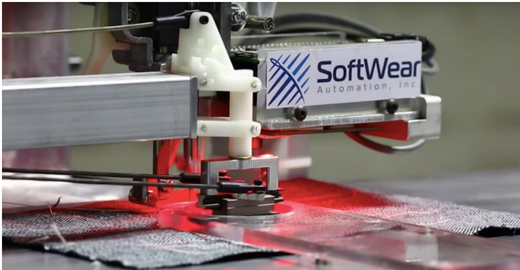
Figure 3: SoftWear's sewing robot that can handle the textile material, position it correctly and sew.
