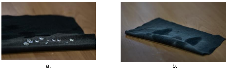
Figure 7. Experiment with water; a. Nano impregnated cotton fabric; b. Non impregnated cotton fabric
