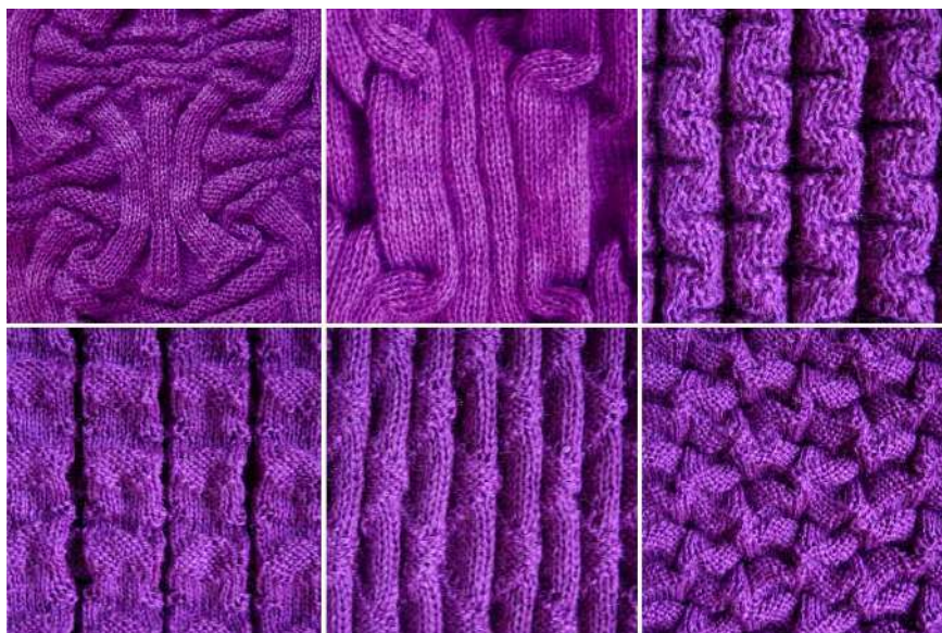
Figure 3. Self-folding links-links structures with different distribution of front and rear loops [5,26]
