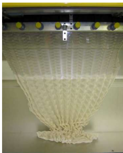
Figure 2. Self-folding of links-links structures after exiting the take-down zone [5]
