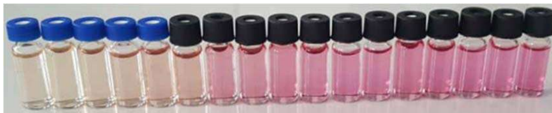
Figure 4. a) UV-Vis spectra of 1 (25 \mu M) upon adding of an increasing concentration of CN - ; b) Photographs of 1 (25 \mu M) with CN - ranging from 0- 9000 Equiv. from right to left.
