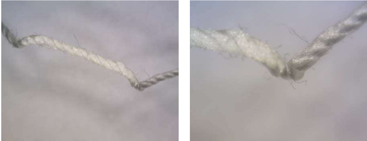
Figure 3. Sewing thread that has suffered major damage after separation from the fabric
