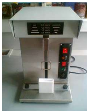
Figure 2. Custom-made apparatus for dip-coating
