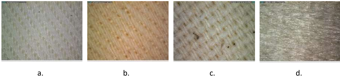
Figure 3. Dino-Lite microscope images of uncoloured textile samples a – white cotton woven fabric (sample 1); b – raw cotton woven fabric (sample 2); c – Panama raw cotton woven fabric (sample 3); d – Velvet fabric (sample 4)
