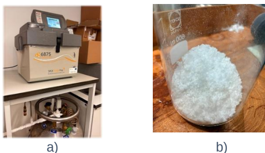
Figure 3: a) Cryogenic mill used for the preparation of the PET internal standard and b) prepared standard particles
