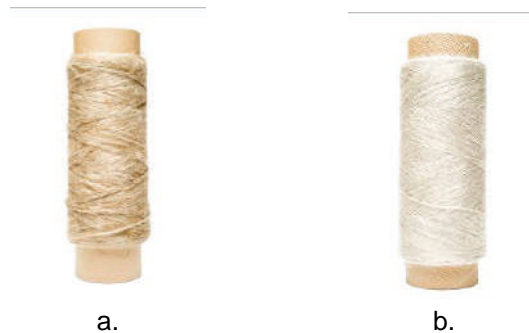
Figure 5: Roving yarns: a. NATTEX ROVING©, Dehondt groupe, 100% flax; b. Roving low twist, Safilin, 100% flax [8]
