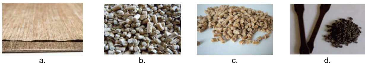
Figure 4: Uni-directional prepreg: a. PROCOTEX, UD flax prepreg, matrix TP and TS; Compound: b. LINCORE CP ©, Groupe Depestele, flax, matrix PVC (polyvinyl chloride), PP (polypropylene), PLA (polylactic acid), ABS ( acrylonitrile butadiene styrene ), PLA recycled; c. AFT PLASTURGIE, hemp, matrix: ABS, PVC, PE (polyethylene), PP; d. ECOTECHNILIN, flax, matrix: PPC (polypropylene carbonate) [8]
