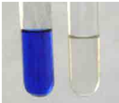
Figure 3: The appearance of C. I. Reactive Blue 19 solution before (left) and after (right) the adsorption of ash, 60 mg/l, at pH 11 and treatment time of 60 minutes
