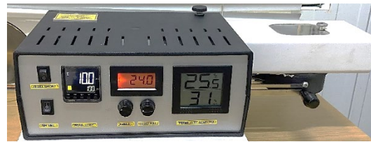
Figure 1: Device for non-destructive measurement of water vapor resistance, Permetest
