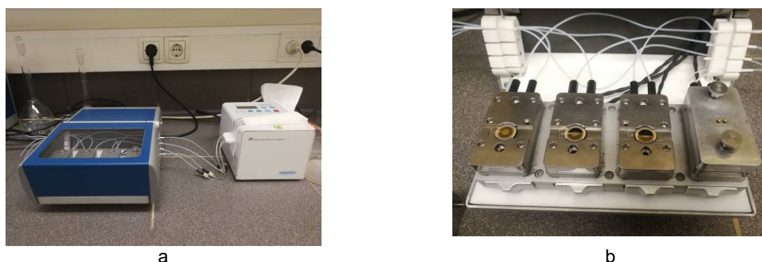
Figure 2: Quartz Crystal Microbalance with Dissipation a) QCM-D b) housing for quartz sensors with cellulose polymer film (MCF).
