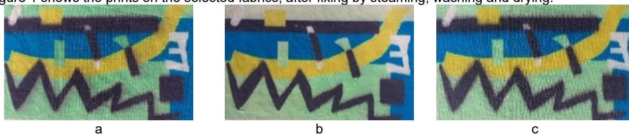
Figure 1: Digital InkJet prints on selected fabrics: a) Plain weave 1/1) b) Twill weave 1/2 Z) c) Atlas weave 1/5
